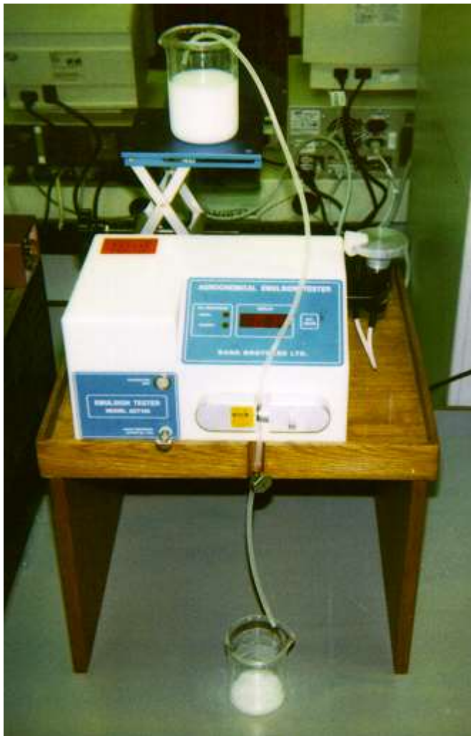
Figure 4 The Agrochemical Emulsion Tester (AET100).
