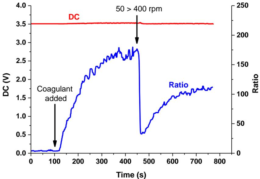
Figure 3 Floc Formation, Breakage and Re-growth—PDA3000 Response
